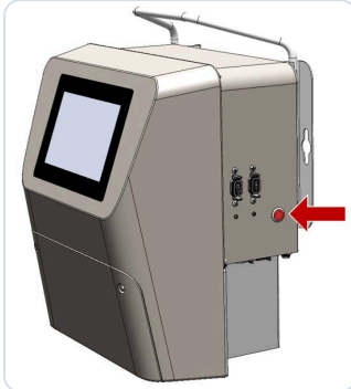
Figure 8-1 Power button of the BactoSense
