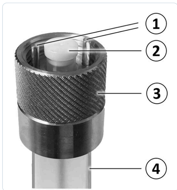
Figure 5-1 Manual sampling device 1: Positioning pins, 2: Plug, 3: Fixation ring, 4: 5 mL screw-cap tube.
